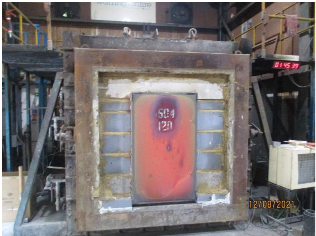
The unexposed face of the steel riser panel after a test duration of 105 minutes
