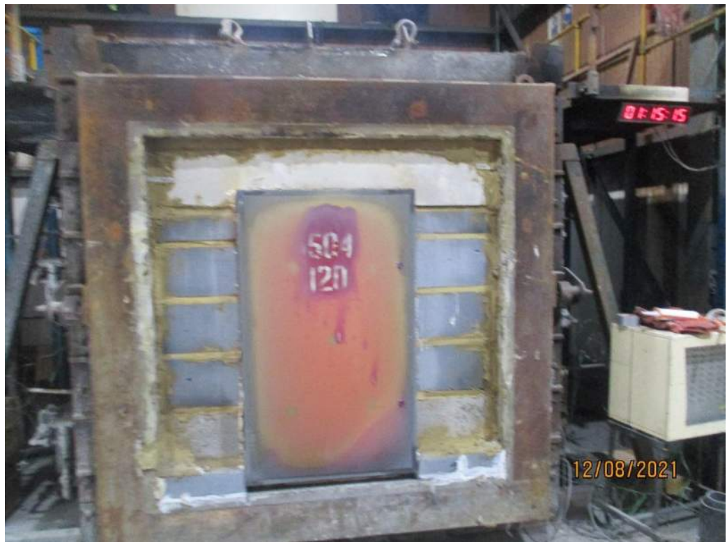
The unexposed face of the steel riser panel after a test duration of 75 minutes
