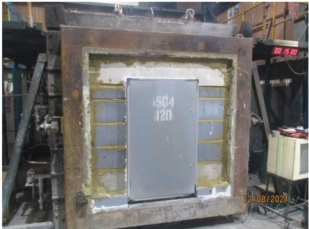
The unexposed face of the steel riser panel after a test duration of 15 minutes
