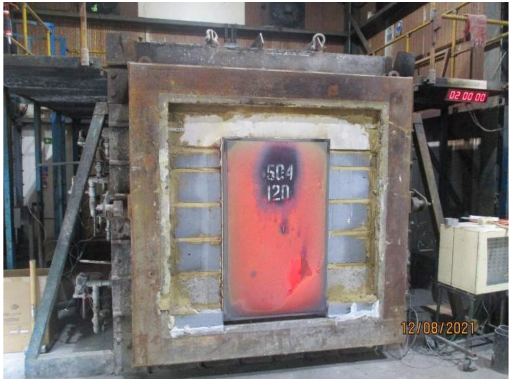
The unexposed face of the steel riser panel after a test duration of 120 minutes
