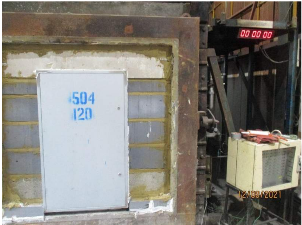
The unexposed face of the steel riser panel prior to testing
