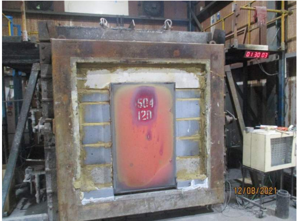
The unexposed face of the steel riser panel after a test duration of 90 minutes
