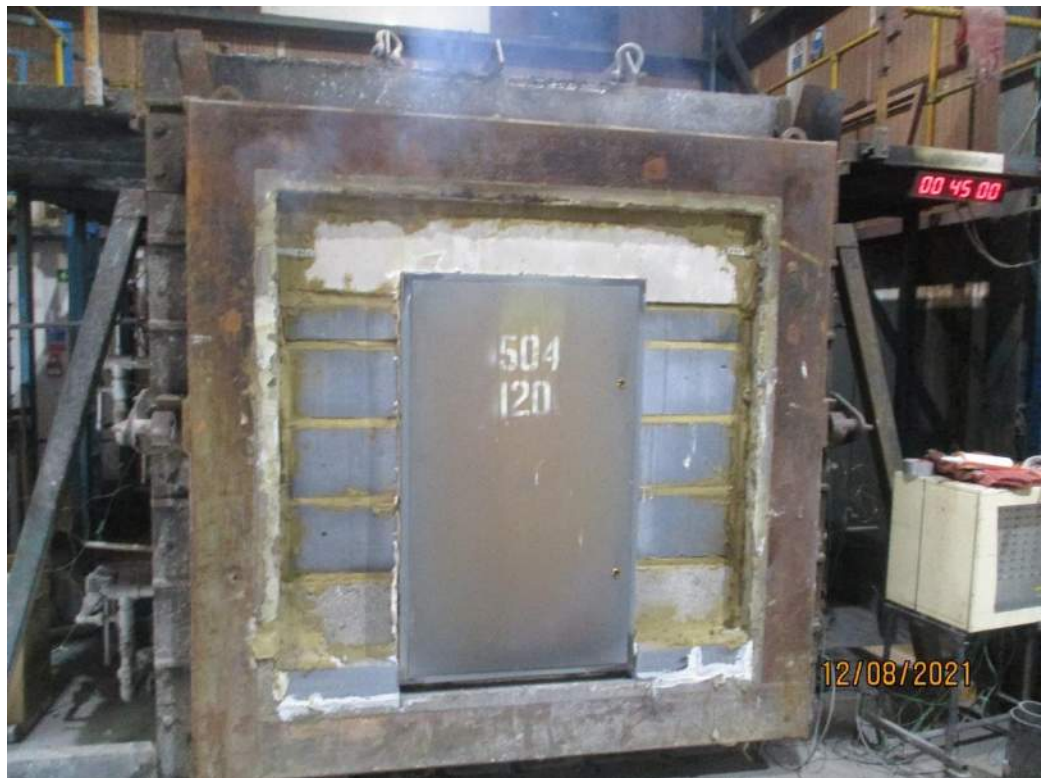
The unexposed face of the steel riser panel after a test duration of 45 minutes
