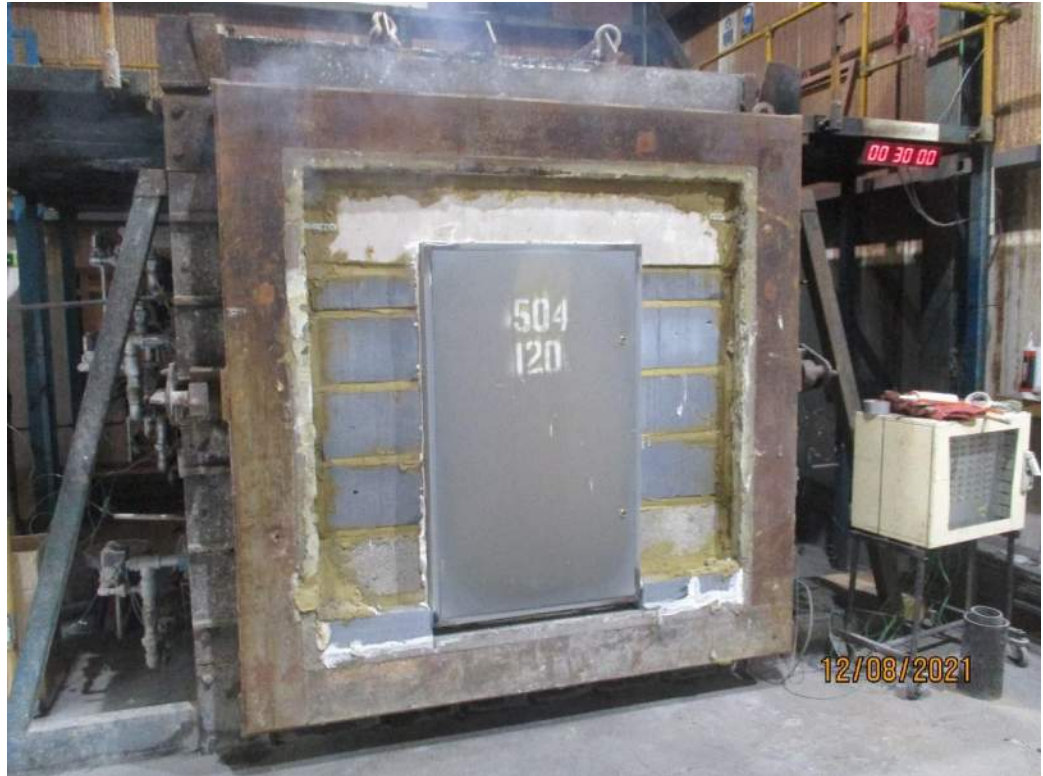
The unexposed face of the steel riser panel after a test duration of 30 minutes
