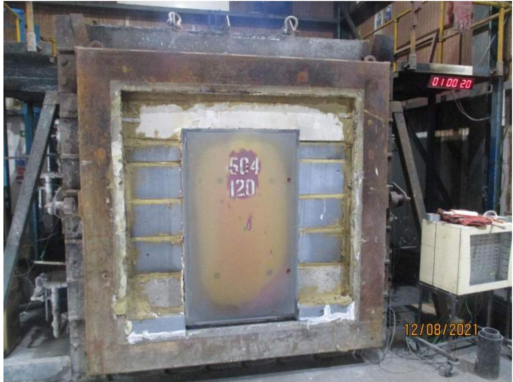
The unexposed face of the steel riser panel after a test duration of 60 minutes
